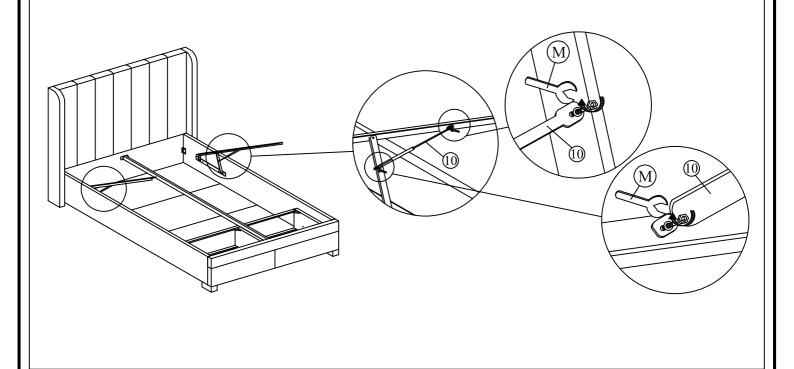
Step 10: Must place the wooden frame (12 & 13) in correct position (please follow the position as shown in diagram).
