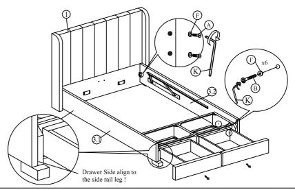
Step 4: Attach the footboard (2) to side rails (3) by pushing the brackets down into place and secure the bolts using hardware part L as shown.
