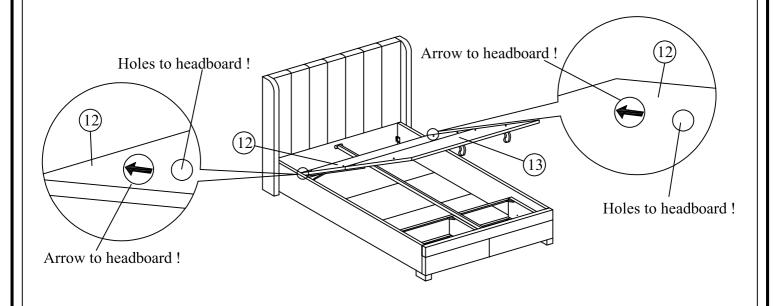
Step 11: Assembly the wooden frame (12) and wooden frame (13) to the bracket and tighten all the fitting accordingly.
