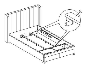
Step 7: Insert the bottom panel (14) to the below frame.
