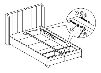
Step 9: Unscrew the Pre-attached hex-nut of gas spring (10) and attach it back again as shown. Please fully tighten the nut.
