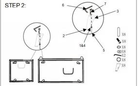
Tighten legs to 80% to start by ALLEN KEY according to the below photo. When all parts have been assembled, you may fully tighten the hardware. To prevent damage to screw threads, do not use a power tool and do not
